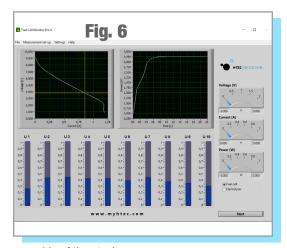
If the measurement bar changes color from blue to red during the measurement, this cell has no power. Among other things, this can be due to insufficient supply of hydrogen or that a water droplet is in the cell which prevents the supply of hydrogen. **Remedy:** check hydrogen supply; blow carefully through the stack; let the stack warm up for some time.
