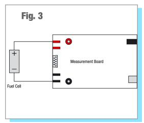
When the program is started, a window is displayed with the instruction to disconnect any possibly connected fuel cells or electrolyzers from the measurement board. This is used for the zero compensation of the FCM. Confirm the by pressing "OK". The FCM is now ready for operation.
